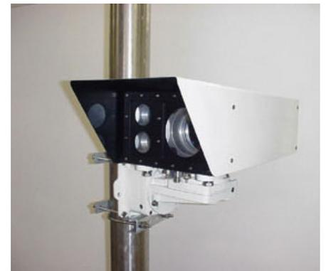
The **Alcatel 9600 FSO** is a SDH/SONET high-capacity Free Space Optics system available in three different versions: SH (Lightweight and very compact for short haul), MH (Very powerful system for medium-haul high-availability links) and LH (Includes a tracking system that supports a very narrow beam width for long-haul links with maximum availability). The Alcatel 9600 FSO is a cost-efficient last-mile solution for Metro Area Network (MAN) providers.
